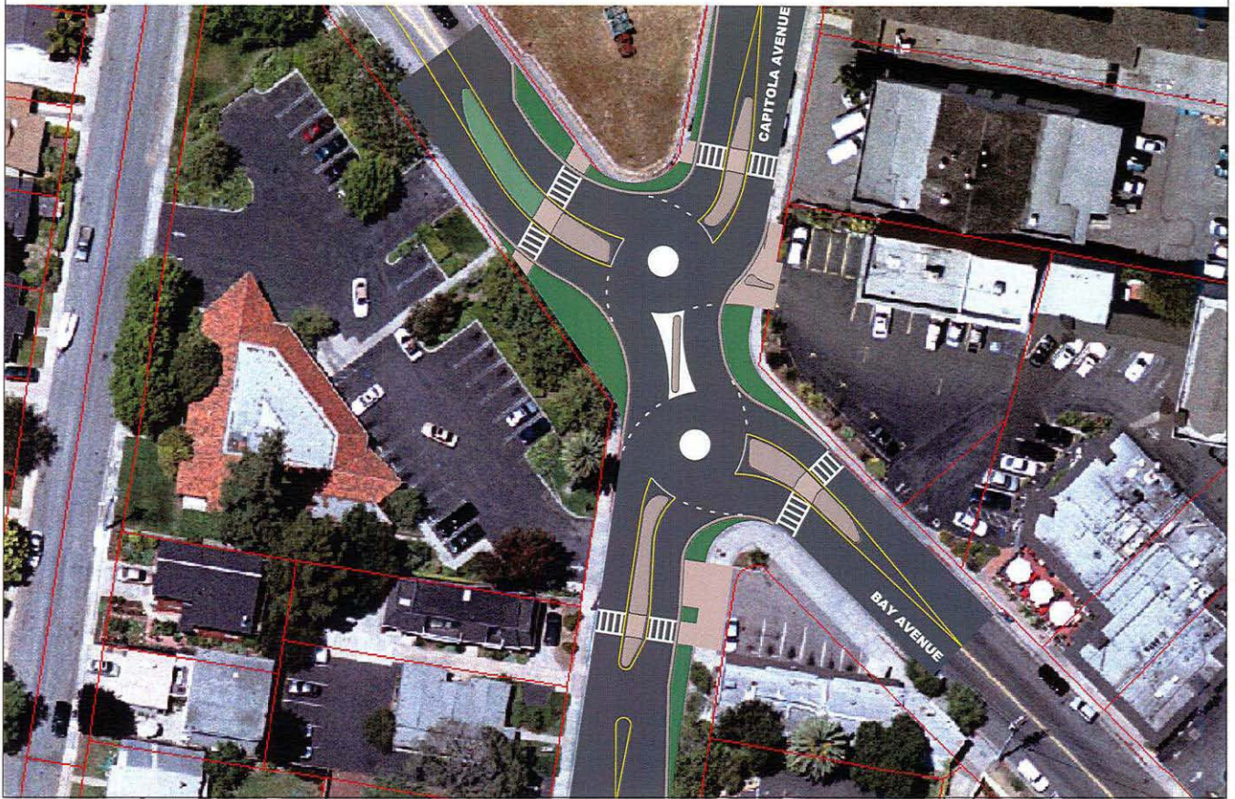
CAPITOLA AVENUE AND BAY AVENUE INTERSECTION CONCEPT 2 - Dual Mini Roundabouts EXHIBIT DM-1 SCALE
