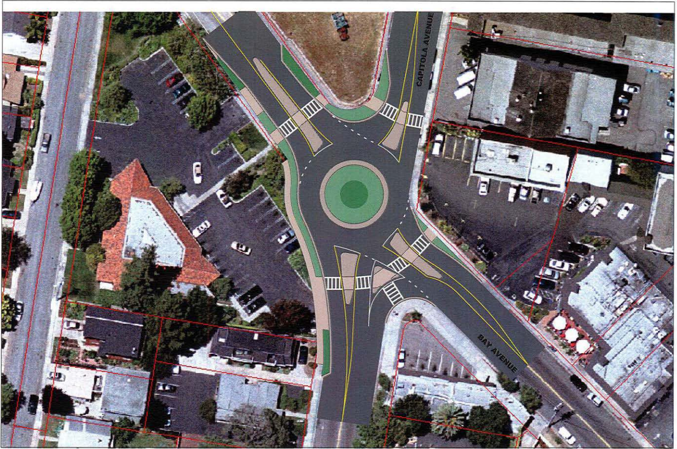
CAPITOLA AVENUE AND BAY AVENUE INTERSECTION CONCEPT 1 - Urban Compact Roundabout EXHIBIT UC-1 SCALE NONE
